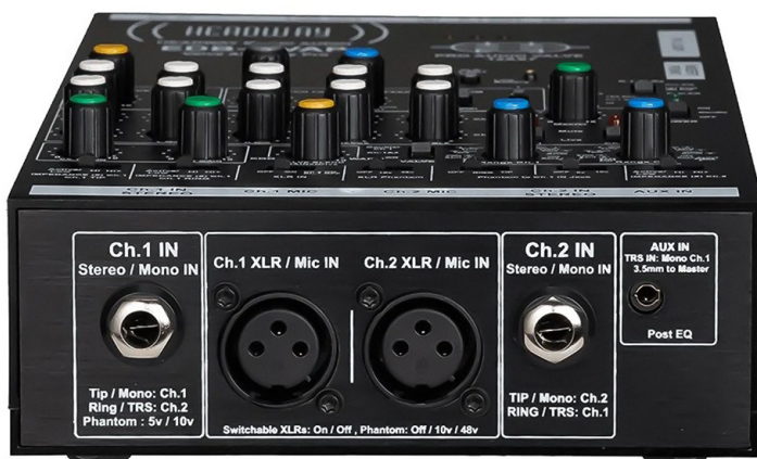
■ The inputs are on the front panel, with the jacks and XLRs supporting different phantom power options.
